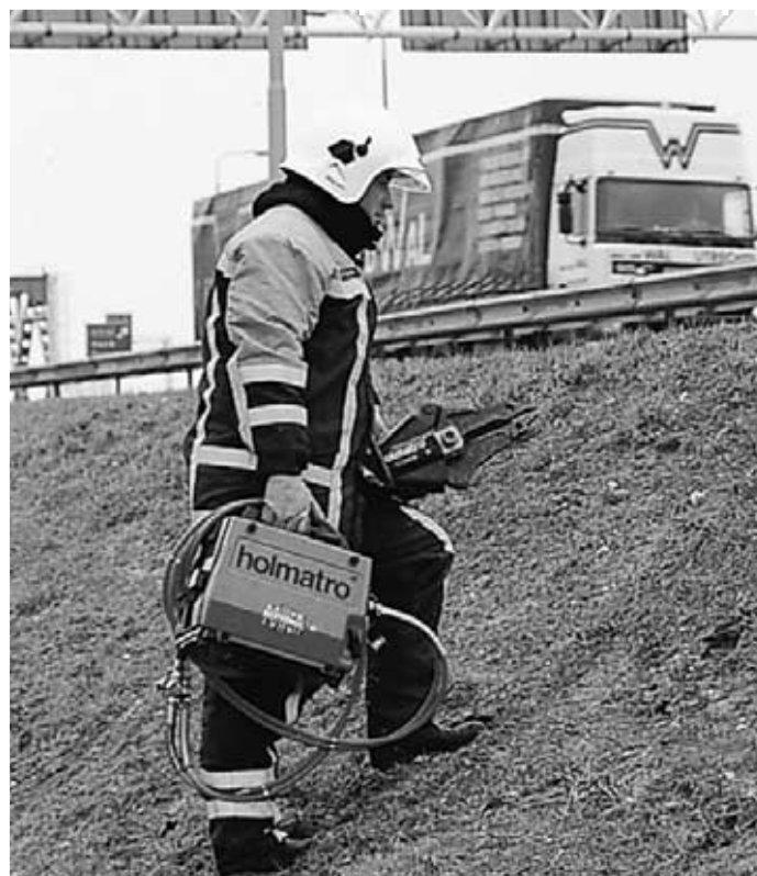
Fig 3. Combined cutting and spreading tool (combination tool) with man portable generator, hydraulic hoses and connectors.
